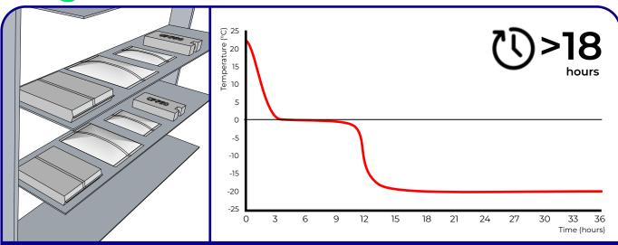
The red line on the graph shows that the temperature of a single coolant pack placed on a shelf in a -20°C freezer went from 22°C to 0°C over a period of 3 hours. The water then went through 'phase change', changing from water to solid. Water-based coolant packs conditioned in single units take up to 18 hours to reach -20°C.
