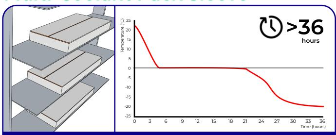
Instead of single coolant packs, some insulated packaging solutions incorporate multi-coolant pack sleeves. In this scenario, where there are multiple coolant packs in each sleeve, freezing time duration is doubled. Water-based coolant packs conditioned in multi-coolant pack sleeves take up to 36 hours to reach -20°C.
