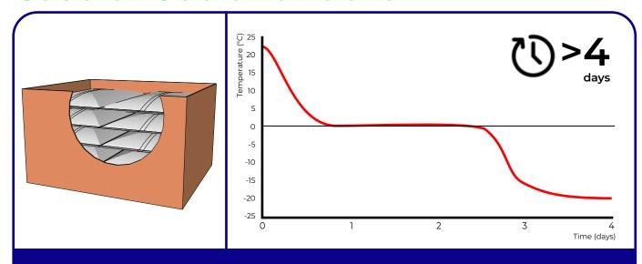
Coolant packs can also be conditioned in multiples, by the case load. In this scenario a case of coolant packs is easily carried from pallet to freezer shelf, and will take several days to reach the required temperature of -20°C. Water-based coolant packs conditioned together in cases take up to 4 days to reach -20°C.
