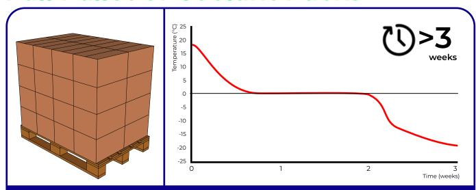
In the event of larger distribution requirements you may need to freeze a full pallet of coolant packs at the same time. This scenario has very important implications on your logistics planning, requiring many weeks to condition a pallet-load of coolant packs. Water-based coolant packs conditioned as a full pallet-load take up to 3 weeks to reach -20°C.
