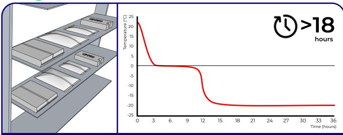
The red line on the graph shows that the temperature of a single coolant pack placed on a shelf in a -20°C freezer went from 22°C to 0°C over a period of 3 hours. The water then went through 'phase change', changing from water to solid. Water-based coolant packs conditioned in single units take up to 18 hours to reach -20°C.
